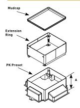
Attaches to preset to add height to preset. Can be field installed.
