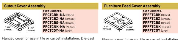
Flanged cover for use in tile or carpet installation. Die-cast aluminum assembly. Provided with one 1" trade size screw plug for power or communication type cabling and one combination 1 1/4" and 2" trade size screw plug for communication type cabling. Allows for feeding both power and communication cabling.
