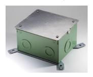
For carpet, tile and wood covered floors. For use in on-grade and above-grade concrete floor applications. Box is provided with a protective, disposable cover that allows the box to be installed at any point in the construction process. Box is available with an epoxy coating for on-grade applications. Custom options are available upon request.
