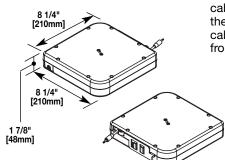
Cable Retractor with 3.5mm Audio cable – Cable Retractor with 3.5mm audio cable. Mounts directly to the InteGreat Series A/V Table Box or to the underside of the conference room table using the TBCRHMK. Loaded with 12' [3.66m] of audio cable that extends out 5' [1.52m] from the retractor. Retractor has a female input from building infrastructure, and a male connector on the output side.
