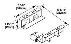
**Cable Retractor Horizontal Mounting Bracket** – Allows retractor to mount horizontally under a conference room table, so cable can be accessed through a table grommet. Multiple retractors can be mounted to each other by attaching the TBCRHMK Mounting B rackets to each other.
