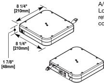
Cable Retractor with Category 6 cable – Mounts directly to the InteGreat Series A/V Table Box or to the underside of the conference room table using the TBCRHMK. Loaded with 12' [3.66m] of Cat6 cable that extends out 5' [1.52m] from the retractor. Retractor has a female input from building infrastructure, and a male connector on the output side.
