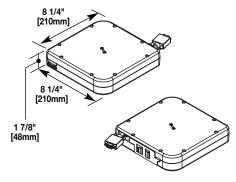
Cable Retractor with VGA cable – Mounts directly to the InteGreat Series A/V Table Box or to the underside of the conference room table using the TBCRHMK. Loaded with 12' [3.66m] of VGA cable that extends out 5' [1.52m] from the retractor. Retractor has a female input from building infrastructure, and a male connector on the output side.
