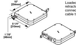
Cable Retractor with HDMI cable – Mounts directly to the InteGreat Series A/V Table Box or to the underside of the conference room table using the TBCRHMK. Loaded with 12' [3.66m] of HDMI cable that extends out 5' [1.52m] from the retractor. Retractor has a female input from building infrastructure, and a male connector on the output side. Input side has mounting tab that allows installer to cable tie HDMI to the retractor to minimize chances of a loose connection.
