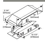
Divided four-gang device box. Allows multiple services (power, data, A/V) at a single point-of-use. Side facing device mounting provides low profile, with space for large cable bend radius. Accepts OFR Series device plates. Removable divider can be aligned with any of the raceway channels.
