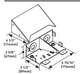
Feeds OFR Series Raceway, Has two (2) concentric 1/2" and 1 1/4" trade size KOs on end. Includes removable divider that can be positioned to feed any raceway channel. Can be used to feed raceway from wall or into furniture.
