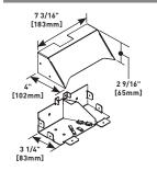
For connecting vertical runs of 2400 & 2400D Series Raceway with OFR Series Raceway. Includes removable divider than can be positioned to feed any raceway channel.
