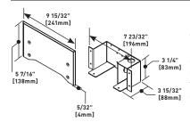
Feeds OFR Series Overfloor Raceway from behind wall. Configurable to provide one or two channels of power. Has 1/2" trade size KO for single channel and 3/4" trade KO for two channel.
