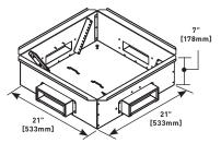
Enclosure for 8" deep floor. Two pairs of pivoting mounting rails for 19" patch panels. Rails support 4 RMU each.
