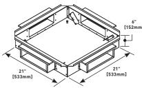
Enclosure for 6" deep floor. Two pairs of rails for 19" patch panels. Rails support 2 RMU each.
