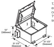
12' deep patch panel enclosure for 2' x 2' drop ceiling tile. One bracket for 19" patch panels. Bracket supports 5 RMU.
