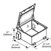
12" deep termination block enclosure for 2' x 2' drop ceiling tile. One removable mounting plate for two 300 pair 1100 style termination blocks (without legs).
