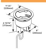
Portal has 9 1/4" [235mm] cover with two (2) duplex receptacles and six (6) Ortronics® category 6 RJ45 jacks and can accept up to ten (10) Legrand AVIP plates or Extron® Electronics MAAP device plates. Units are prewired with 12' [3.7m] cord with NEMA 5-15P plug and are available with die-cast aluminum cover with durable powder coat finishes of nickel (WS8FNK), bronze (WS8FBZ), gray (WS8FGY), black (WS8FBK), or brass (WS8FBS).
