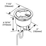
Portal has 7 1/4" [184mm] cover with two (2) duplex receptacles and two (2) Ortronics® category 6 RJ45 jacks and can accept up to five (5) Legrand AVIP plates or Extron® Electronics MAAP device plates. Units are prewired with 12' [3.7m] cord with NEMA 5-15P plug and are available with die-cast aluminum cover with durable powder coat finishes of nickel (WS6FNK), bronze (WS6FBZ), gray (WS6FGY), black (WS6FBK), or brass (WS6FBS).
