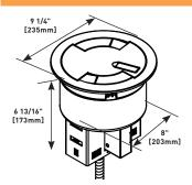
Portal has 9 1/4" [235mm] cover with two (2) duplex receptacles and six (6) Ortronics® category 6 RJ45 jacks and can accept up to ten (10) Legrand AVIP plates or Extron® Electronics MAAP device plates. Units have 6' [1.8m] whip for field-wiring and are available with die-cast aluminum cover with durable powder coat finishes of nickel (WSF8FNK), bronze (WSF8FBZ), gray (WSF8FGY), black (WSF8FBK), or brass (WSF8FBS).
