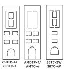
Communication covers for additional voice/data connectors. Each cover includes KOs for four RJ11/RJ45 connectors (.760" x .576" [19.3mm x 14.6mm]), mouse hole for exiting communication cables (grommet furnished).
