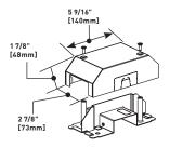
Allows 2400 Series Raceway runs to bridge over existing installations of 2400, 500, and 700 Series Raceways.
