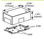
Connects existing installations of 2100 Series Raceway to 2400 Series Raceway.
