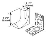
Eliminates need to offset 2400 Series Raceway when connecting with surface panel boxes. Has 3/4" and 1" concentric trade size KOs with 1" trade size KO elongated so adjustment from surface to center of bushing is 1" [25mm] minimum to 1 5/8" [41mm] maximum. Has twistouts
