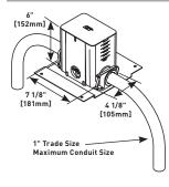
Box comes complete with reusable mudcap, insert spacer, conduit plugs and reducers. Reducers provided for reduction to 1", 3/4", and 1/2" [25mm, 19.1mm, and 12.7mm] conduit. Minimum concrete depth is 3 1/2" [89mm] and maximum concrete depth is 6" [152mm]. Minimum capacity is 50 cu. in. [819ml] and maximum capacity is 100 cu. in. [1639ml]. Box dimensions are 4 1/8" W x 5 1/2" L x 6" [105mm x 140mm x 152mml.
