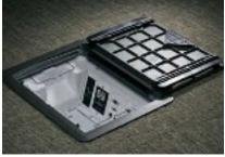
**Durable 180° Articulating Hinge** Hinge design enables covers to open a full 180° and lie flat on the floor surface with the durability to support a large cover. Provides easy access to all interior modules and activations while reducing tripping hazards.
