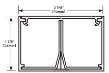
AL3300 Series Raceway's low profile, divided aluminum raceway meets the demands of today's laboratories, healthcare facilities and upscale office locations, providing a compact and effective method of consolidating power and communication cabling.
