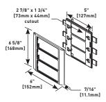
For mounting up to three power and communication devices with the 5500 Series Raceway. Utilizes 5507 Series™ Faceplates, Wiremold Open System communication modules, Ortronics® TracJack and Series II inserts, and Pass & Seymour® Activate Series inserts. For faceplate options, see 5507 Series™ Faceplates. Available in ivory (5550) and white (5550-WH).
