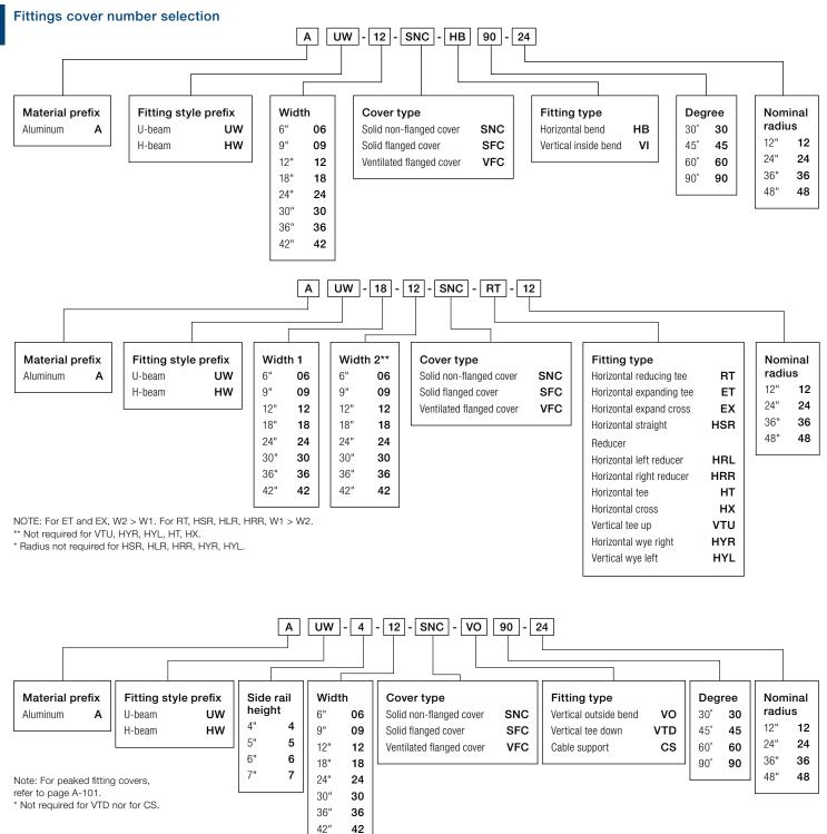
T&B aluminum cable tray is composed of two distinct systems, H-style and U-style. These systems are interchangeable.
