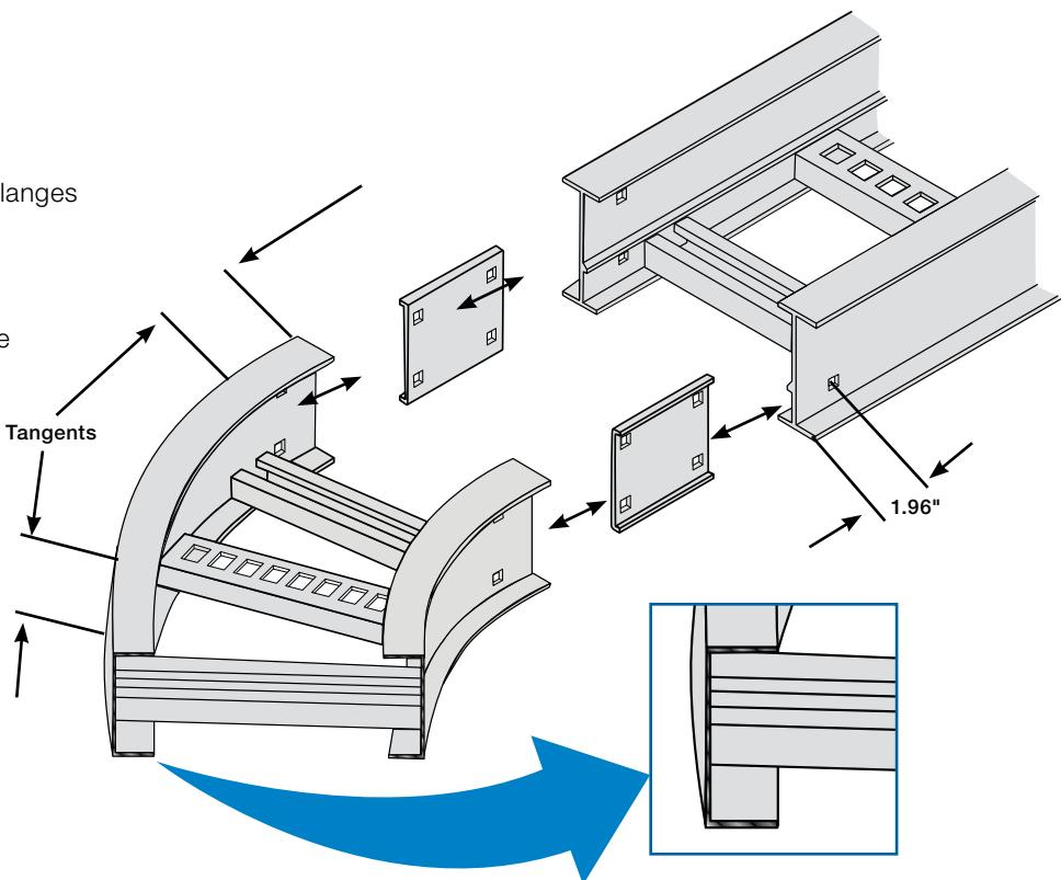
T&B aluminum cable tray is composed of two distinct systems, H-style and U-style. These systems are interchangeable.
