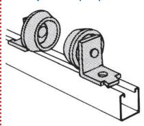
Cast aluminum rollers, steel brackets. Designed for standard saddles. Order separately for each pair of rollers: two 1/2 in. x 5/16 in. hex head cap screws and two 1/2 in. channel nuts. Space to suit 0.D. of pipe and wrapping.
