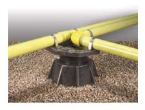
The T&B Adjustable Universal Support (AUS) provides an easy method for supporting pipes, conduit and equipment on flat roofs, below raised floors and even on level ground applications. The AUS reduces installation time compared to other support solutions such as wooden blocks, cement blocks, straps and clips. These labor intensive solutions also increase the danger of roof membrane penetration.
