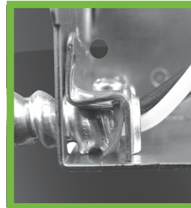
The "LA" cable clamp has been designed so that the anti-short bushing and the armour butt-up against a retaining wall built into the clamp
