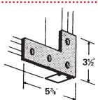
Standard Dimension Hole Spacing Hole Spacing Hole Size Material Material 13/16 in. From End 1-7/8 in. Centers 9/16 in. Diam. 1-5/8 in. Width 1/4 in. Thick
