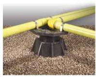
The T&B Adjustable Universal Support (AUS) provides an easy method for supporting pipes, conduit and equipment on flat roofs, below raised floors and even on level ground applications. The AUS reduces installation time compared to other support solutions such as wooden blocks, cement blocks, straps and clips. These labor intensive solutions also increase the danger of roof membrane penetration.
