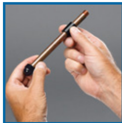
3. Remove one end nut and spacers from Multi-Tap rod.
