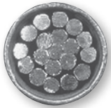
Before compression, a typical cross section of cable and connector consists of about 75% metal and 25% air.
