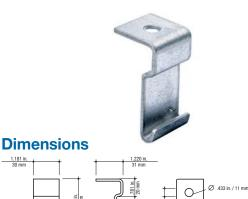
The side hanger clamp is used to construct trapeze supports using threaded rods. The offset support hole allows for trouble-free access to support nuts for height adjustment and the rod can continue downward to allow for multi-level (tiered) trapeze installations. A set screw holds tray firmly in position once installation is complete. Available in pregalvanized steel. For use with 3/8 in. threaded rod.
