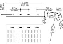
For larger cable tray widths and heavier cable loading, use the 7 in. radius large cable drop-out to protect cable exiting or entering tray runs. Available in pregalvanized steel, the large cable drop-out has a versatile slotted design that enables the use of Ty-Rap® cable ties to attach the cable bundles to the drop-out.
