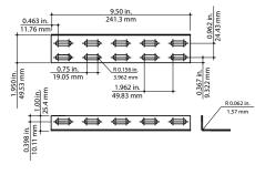
Support and terminate runs of cable tray with this wall termination angle. Can be used as a wall support, floor to ceiling support or to safely terminate any tray run. Adapts to any configuration and any width. Available in pregalvanized steel. Mounting hardware sold separately.
