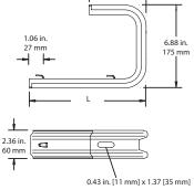
The "J" bracket with TabLok™ profile provides a secure attachment surface requiring no additional hardware for mounting ExpressTray® to ceilings. This bracket is available in 6 in., 8 in., 10 in. and 14 in. lengths to accommodate wire basket profiles up to 12 in. wide and 4 in. high. Available in pregalvanized steel.
