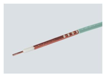
The RCoax cables are radiating cables that function as special antennas for the SCALANCE W Access Points in environments with complex radio coverage. Its design means that a defined, cone-shaped radio field is generated along the RCoax cable. The radiating cables are therefore perfectly suitable for use in all types of applications with track-bound vehicles.
