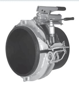
If the end of a PE pipe is not perfectly round, the coupling will not fit over the end of the pipe. Our Re-Round Clamps solve this problem.
