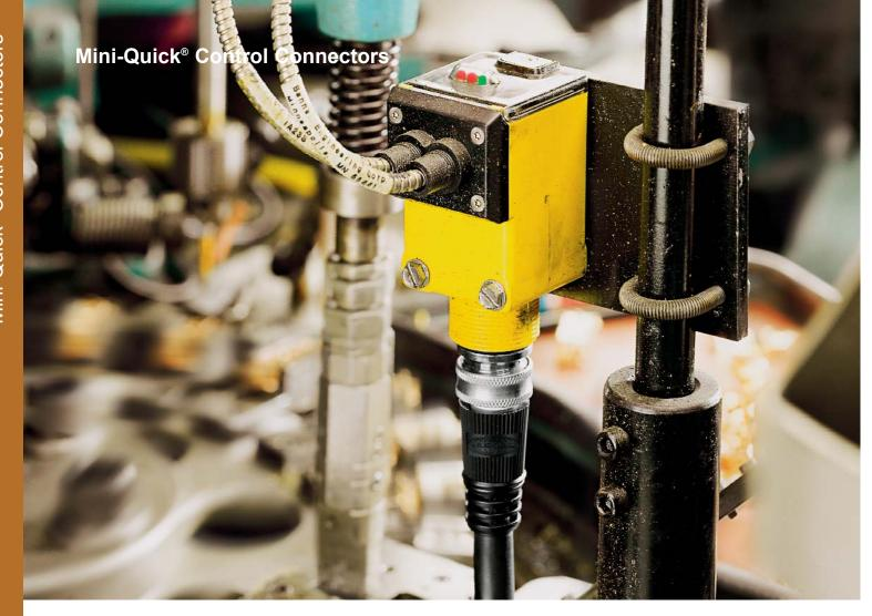
Mini-Quick Control Connectors are a line of environmentally protected, industrial circular connectors typically used for the installation and quick disconnect of solenoid valves, photo eyes, limit switches and 18 and 30 mm proximity switches. The electrical and environmental ratings of Mini-Quick connectors also make them well suited for use with outdoor lighting as well as other commercial applications requiring circular disconnect cable assemblies.
