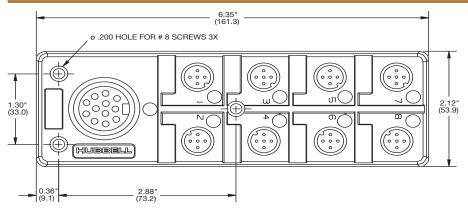
\* Hard wired and connectorized enclosures have same enclosure dimensions.
