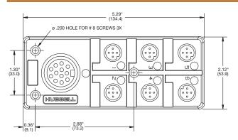
\* Hard wired and connectorized enclosures have same enclosure dimensions.
