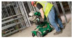
Switching the 855GX between vertical and horizontal bending configurations is simple and can be done in seconds with its unique pivoting cylinder.
