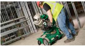
Switching the 855GX between vertical and horizontal bending configurations is simple and can be done in seconds with its unique pivoting cylinder.
