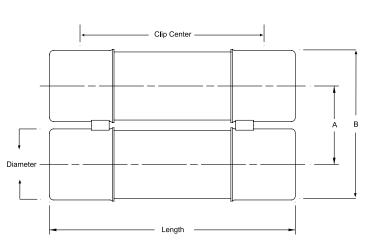
9F series A = 3.31 inches (84mm) 9F series B = 6.16 inches (160mm) Amp-Trap series A = 3.63 inches (92 mm) Amp-Trap series A = 3.63 inches (169 mm)
