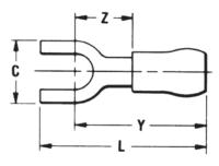
NOTE: Field bending straight lugs to achieve an angular connection will void UL Listing / CSA Certifications and BURNDY will not be liable for the connection.
