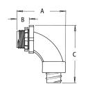
For use with non-metallic liquid-tight conduit, type B only. Produced from UV rated plastic for long outdoor life.
