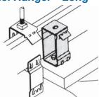
Illustration showing A854L with nut and bolt furnished to attach to fluorescent fixture. Use with E and H Series channel as well as A, B, C or D Series channel. Wt./C 51 lb.
