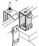
Illustration showing A854 with nut and bolt furnished to attach to fluorescent fixture. Use with A. B. C or D Series channel. Wt./C 34 lb.
