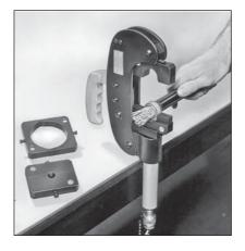
All the 2-piece Shield-Kon® in the circular range need to be crimped with the 13640 hydraulic head equipped with the appropriate die.
