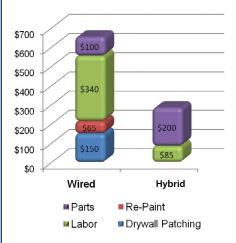
\*Installation time per device: 45-50 minutes for hardwire vs. 10-15 minutes for wireless devices.
