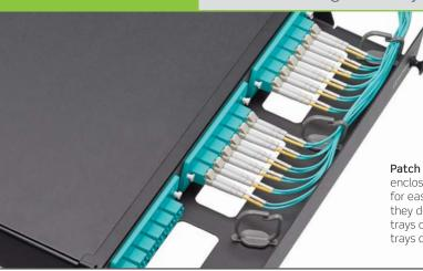
**Patch Cord Management Trays** help route and organize cables on 500i SDX enclosures. The trays feature identification labels and front saddles that pivot for easier routing. Because they mount directly to the front of the enclosures, they do not require additional rack space. Available in 1RU and 2RU sizes, the trays can be used with any Leviton 1RU flush-mount MTP enclosure, and 2RU trays can be used with 3RU 500i SDX enclosures. (See page B29.)
