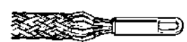
Rotating Eye For use in changing wire rope in large cranes and derricks.
