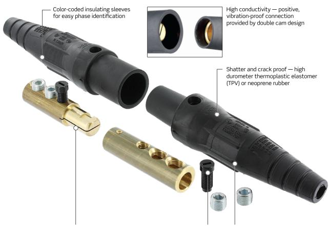
Self compensating for wear slit and cam in male contact provides spring action for longer usage
