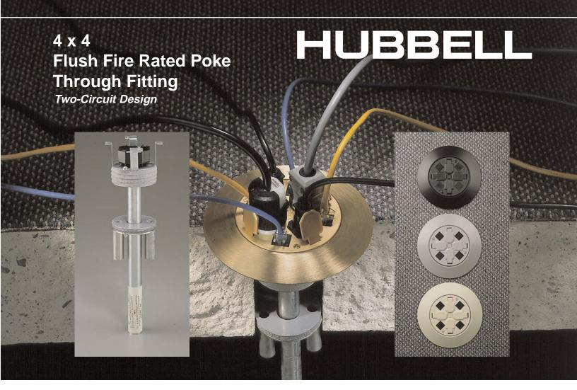
Hubbell introduces a multiple service fire rated poke through fitting that combines four insulated 15 ampere, 125V receptacles with four category 5 jacks to be installed in a 3" cored hole. This additional service capacity provides the maximum in flexibility if requirements change. Four
