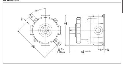
\*Furnished with four \*/4" standard taper tapped, integrally bushed hubs. Each hub as a \*/4" to \*/2" reducer. Three hubs are plugged.
